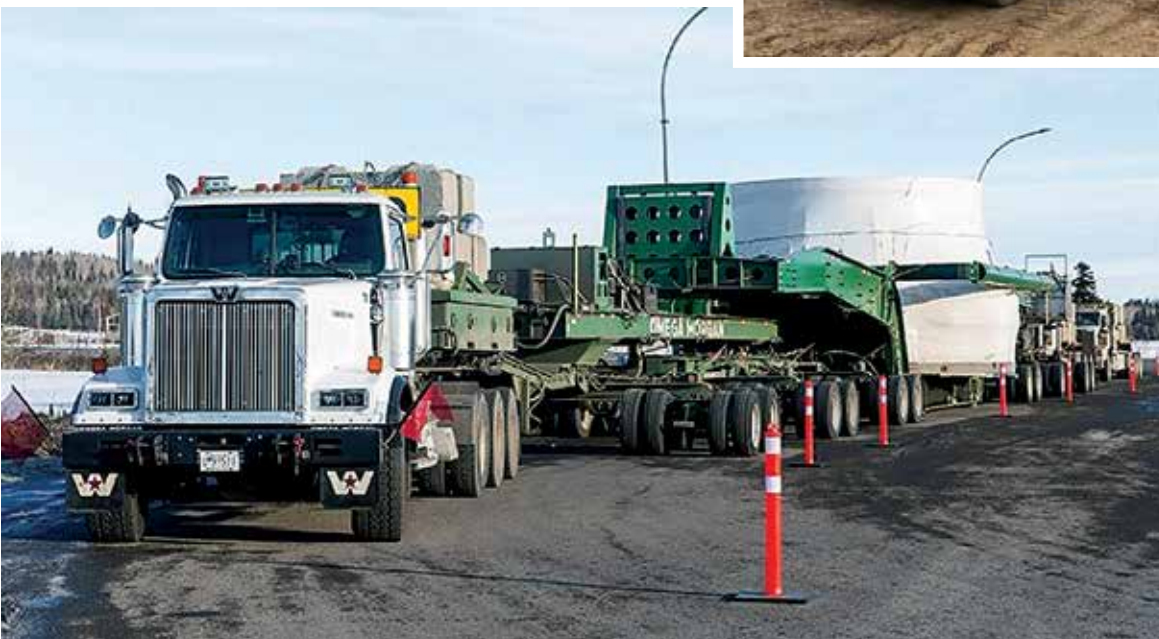
Teamsters Local 213 members carefully move turbine components from Prince Rupert to Site C, where they are housed at Units 1 and 2 inside the Site C powerhouse.
