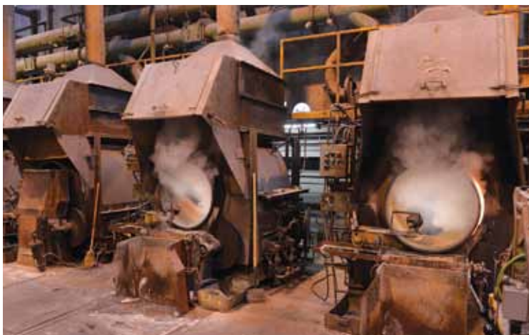
The hot galvanizing ovens where the zinc adheres to the nails.
