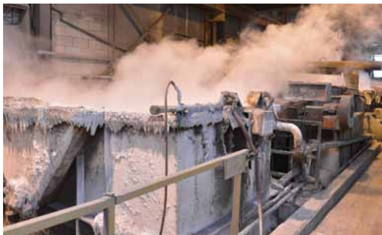
The lime, sulphuric and water baths in the cleaning house.
